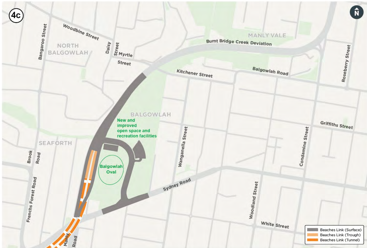
Figure 4-27 Alternative 4c - North facing tunnel ramps to Burnt Bridge Creek Deviation with shortened, centralised access road to distribute traffic and provide connection to the new and improved open space and recreation facilities
