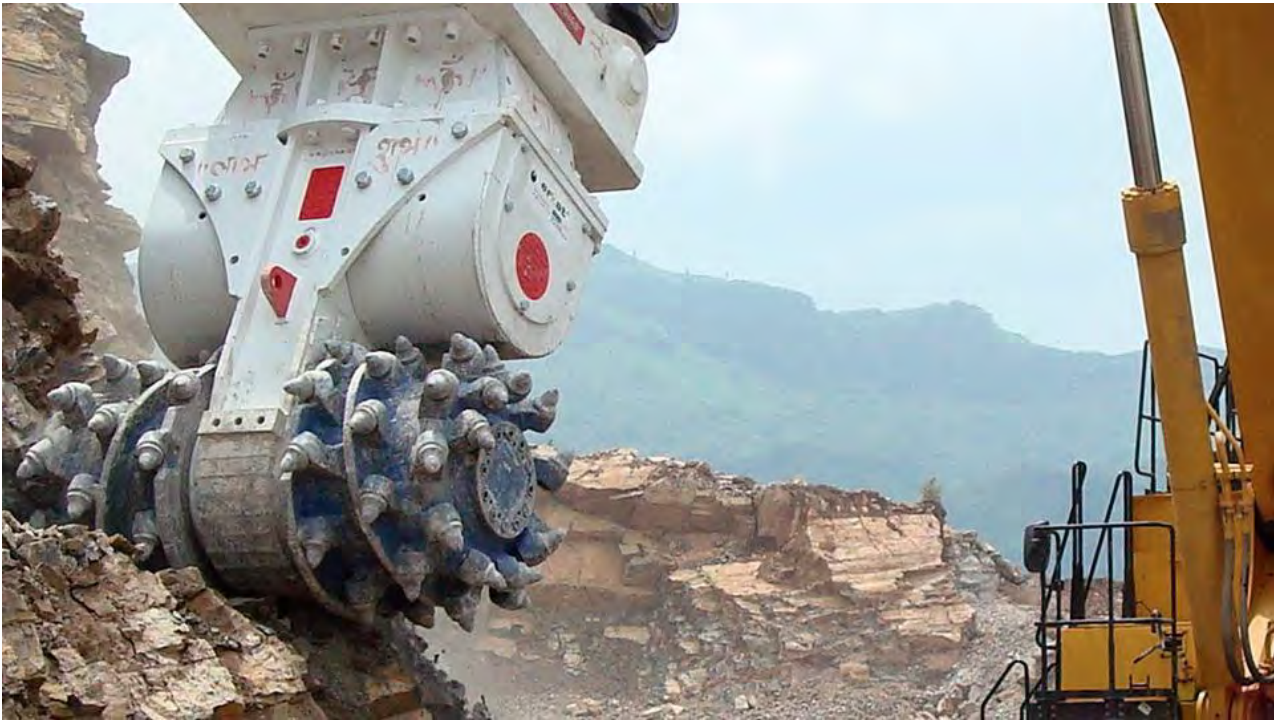
Figure 6-15 Example of drum cutters which can be used in a marine situation
