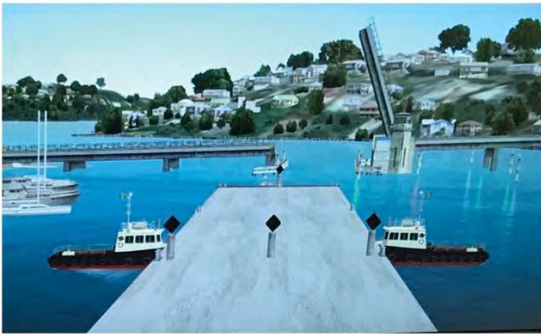
Transport of steel shell units through Spit Bridge.
