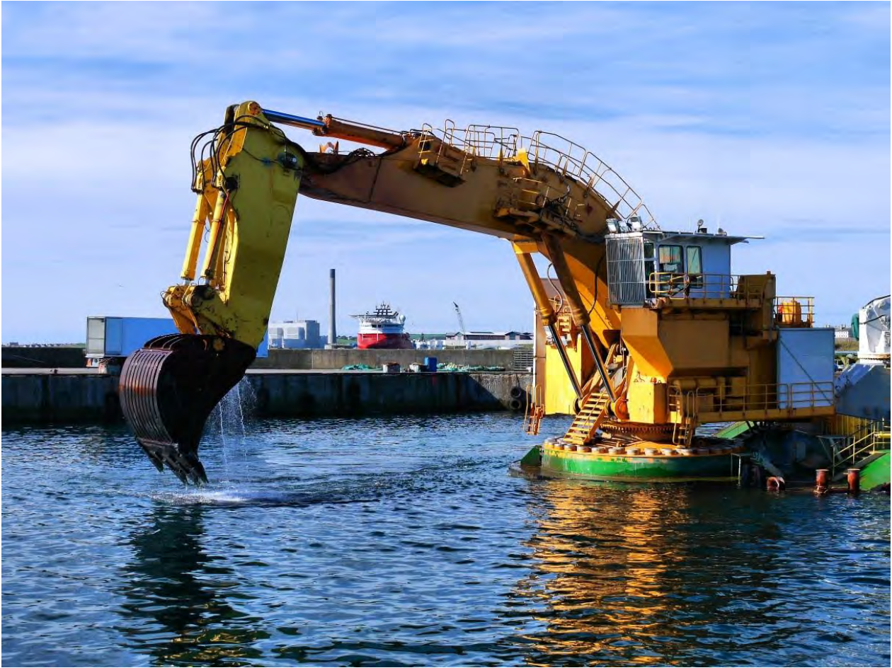
Figure 6-13 Example of backhoe dredger with an open bucket (Royal Haskoning DHV, 2020)
