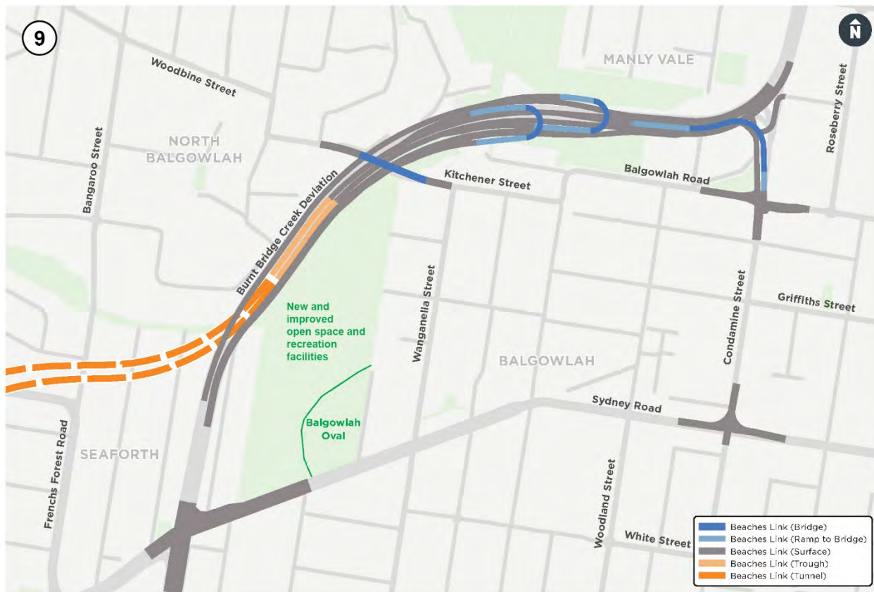
Figure 4-32 Alternative 9 - North facing tunnel ramps to Burnt Bridge Creek Deviation with dual U-turn overpass facility
