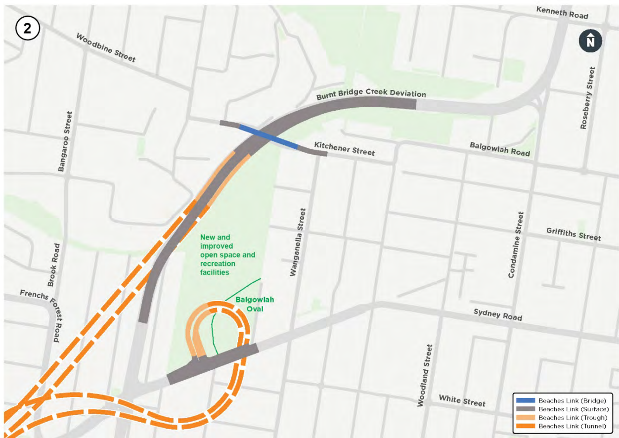
Figure 4-23 Alternative 2 - Tunnel loop ramps to Sydney Road
