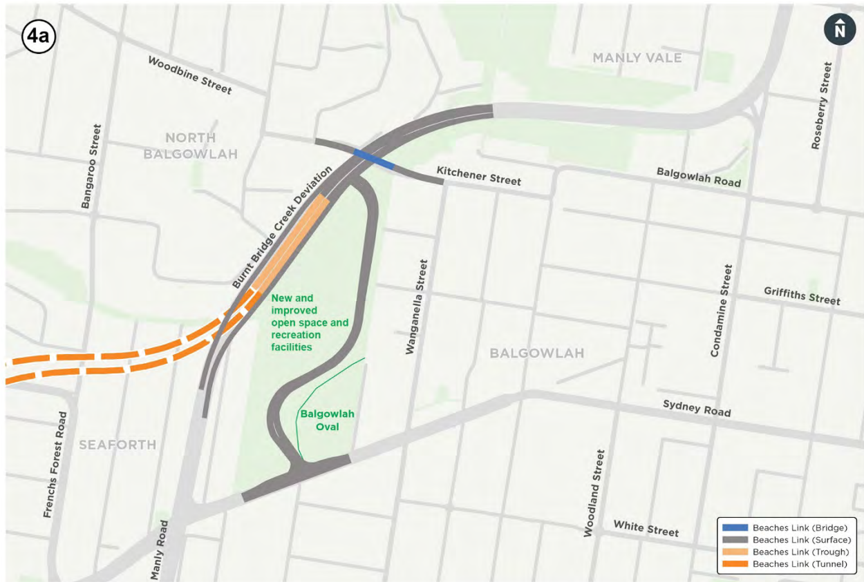
Figure 4-25 Alternative 4a - North facing tunnel ramps to Burnt Bridge Creek Deviation with access road to distribute traffic and provide connection to new and improved open space and recreation facilities
