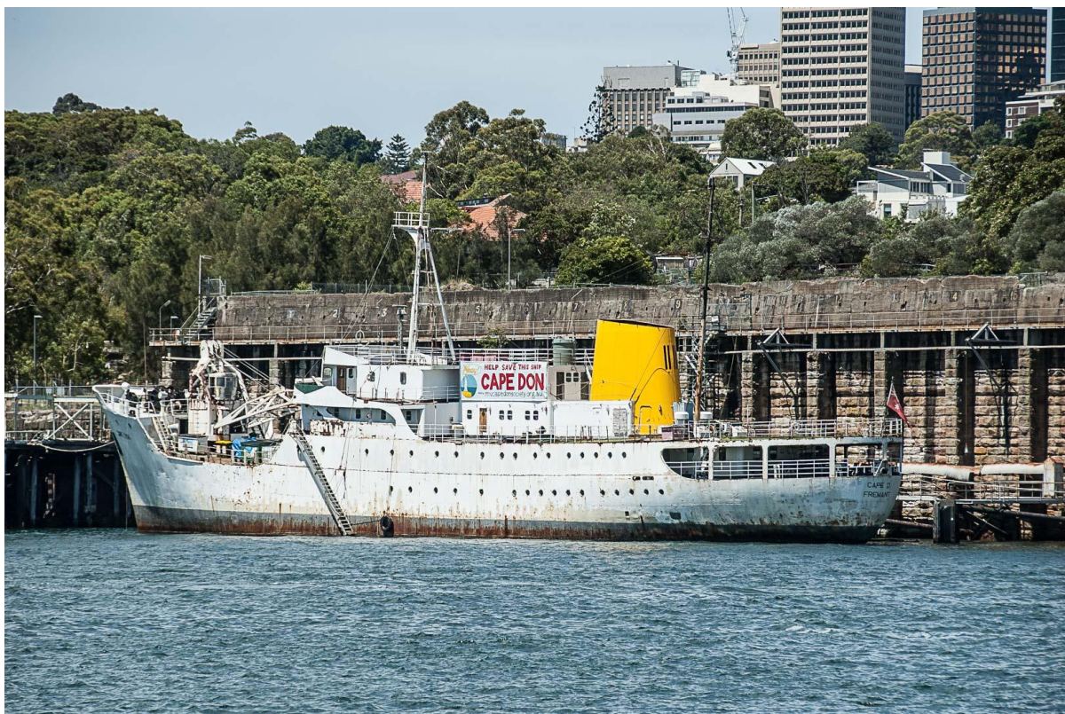
Fig. 8 Cape Don in 26/12/2010 The waterline colour was bright green in 2008 and is now rusted.
